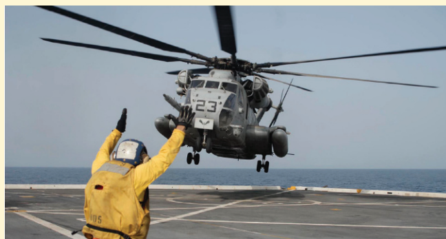
Figure 2 | The CH-53E will soon be outfitted with a Guardian laser transmitter assembly. U.S. Navy photo by Mass Communications Specialist 1st Class Steve Smith
